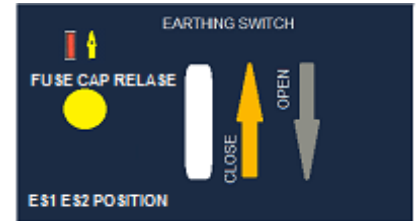
Figure 18 - Mask for the operating point of the transformer unit earthing switches (see table 8 for the correct wording) and for fuse-cover release (to be translated in local languages)
