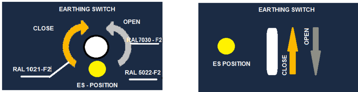
Figure 23 - Mask opening and closing of the earthing switch (see table 8 for the correct wording)
